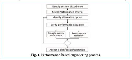
The performance-based water resources engineering process in Figure 1 can be implemented in (i) an iterative way by examining alternative options (plans/designs/operational strategies) ahead of system disturbance or (ii) in real-time by responding to system disturbance and managing recovery from it. Verification of system performance capability is done by the combined use of simulation and quantitative resilience assessment.
